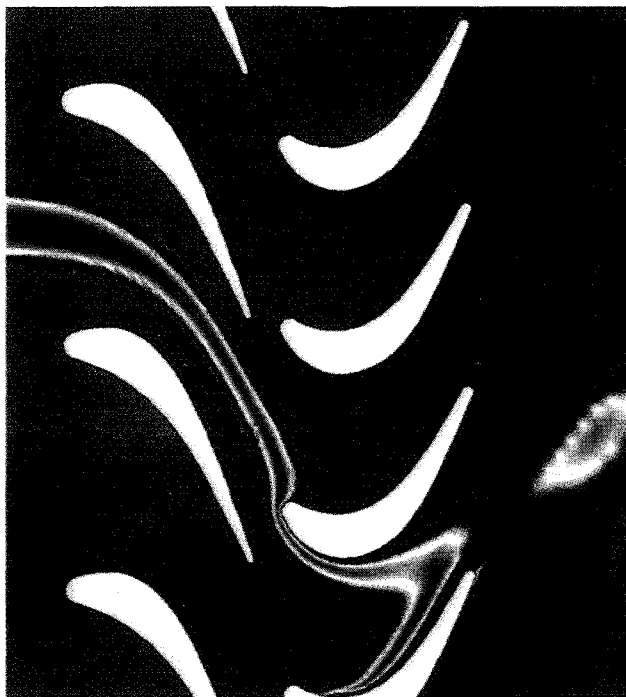
Fig. 5 Static temperature contours for stator base cooling simulations.
